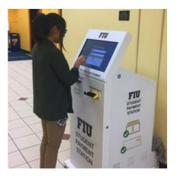
The ADA compliant solution includes a check scanning and escrow device, bill acceptor with bunch note feeder, touchscreen navigation, thermal receipt printer and a camera for added security and analytics.
